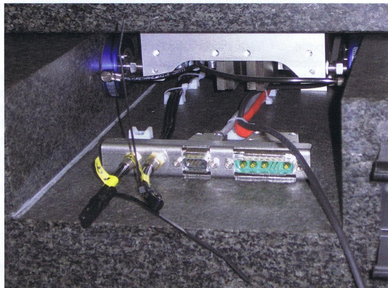
Figure 3. The underside of the lower axis carriage, with guidance air-bearing pucks mounted.
